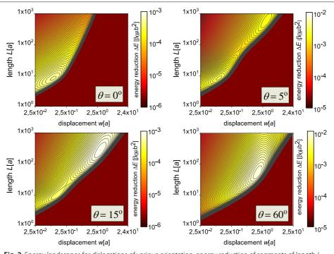
**Fig. 2** Energy landscapes for dislocations of various orientation, energy reduction of segments of length L displacing over the distance w according to Eq. (19), angles are given in the figures
