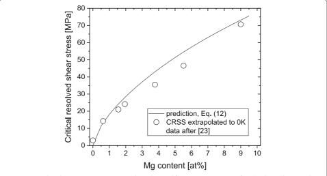
**Fig. 6** Extrapolated zero-temperature CRSS data obtained from measurements of Podkuyko and Pustovalov (Podkuyko and Pustovalov 1978) on  $AIMg_x$  single crystals, and prediction derived from Eq. (12)
