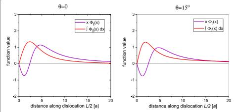
**Fig. 4** Determination of the pinning length for screw-like pinning from Eq. (24) for a pure screw (left) and a 15 deg dislocation (right). Note that Eq. (24) is not valid for the edge-like branch of pinning energy maxima which exhibits much higher pinning displacements
