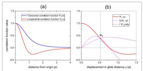
**Fig. 1** (a) Longitudinal and transverse correlation functions of the fluctuating shear stress in an effective medium with random volumetric misfit, blue: transverse correlations, red: logitudinal correlations, (b) determination of the optimal pinning displacement for an edge dislocation from the longitudinal correlation function
