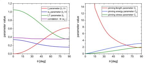
**Fig. 3** Left: Dependence of scaling parameters on dislocation orientation angle  $\theta$ ; right: Corresponding parameters  $C_L$ ,  $C_E$  and  $C_\tau$  which govern the angle dependence of the pinning length, pinning energy and pinning stress, respectively
